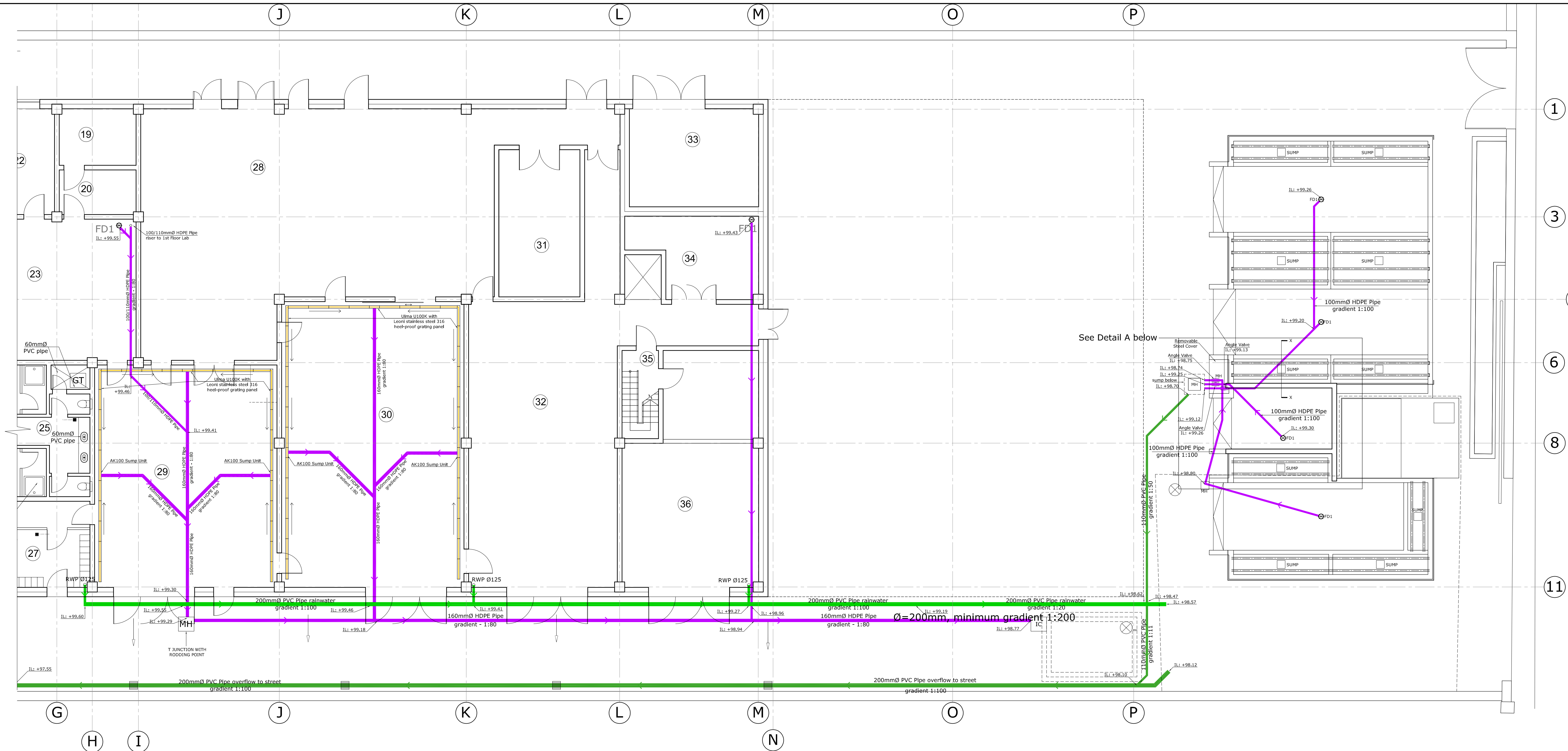
Drainage Layout - Level 0 (Production) scale 1:100
